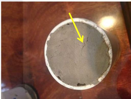
Figure 1 (left). Bottom side of concrete cylinder shows cracks due to sudden loss of water content and thermal shrinkage when simple is irradiated with 6.5 Watts.
