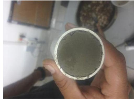
Figure 3 (left). No cracks appear at the top side of the concrete cylinder when the sample is irradiated with 3.5 Watts.
