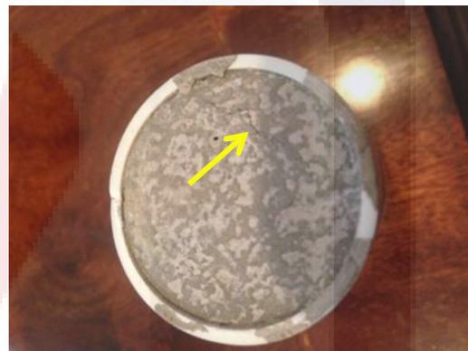
Figure 2 (right). Top side of concrete cylinder shows cracks due to sudden loss of water content and thermal shrinkage when simple is irradiated with 6.5 Watts.
