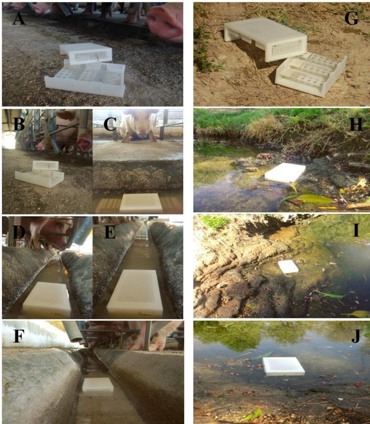
Figure 53: Mobile device for obtaining biofilms directly from the environment. The device can be placed in a great number of places where you want to get the environmental biofilm.
