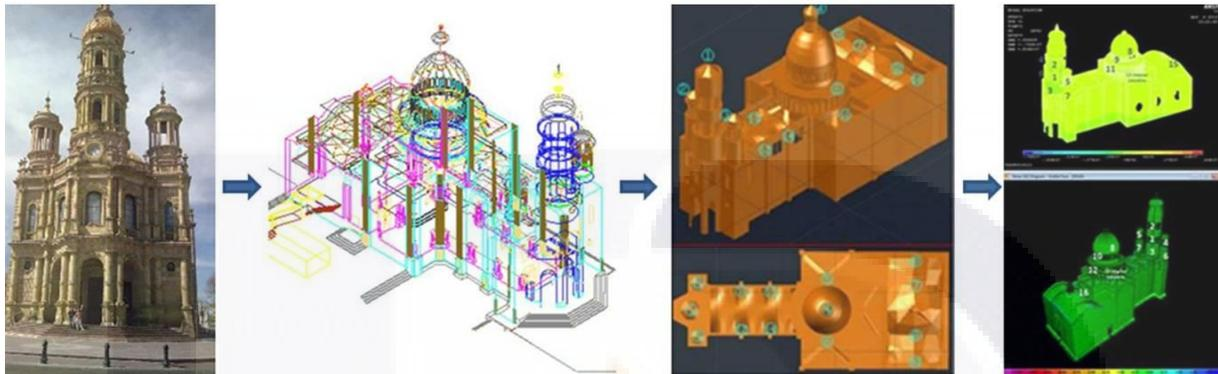
Figure 1. First approach to the structural condition of the Temple with SAP2000.
