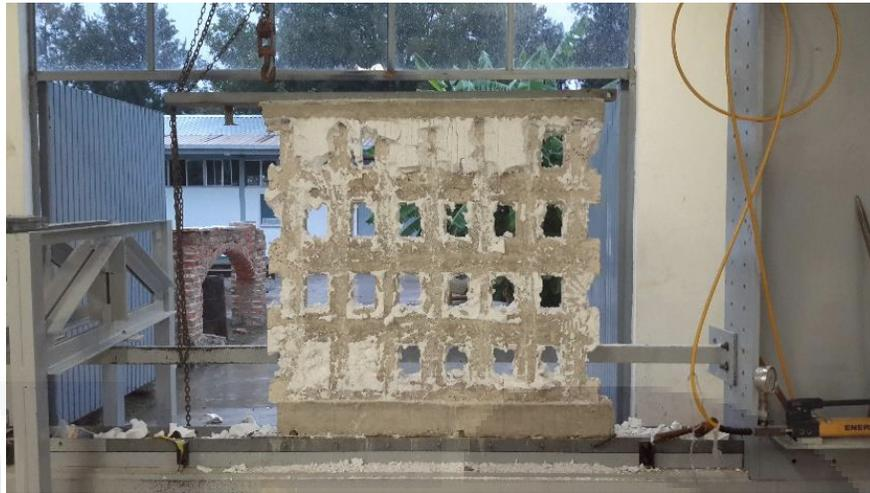
Figure 3. EPS removal from the wall.
